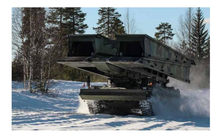
The LEGUAN is a modular, versatile and extremely powerful overall concept for the fast and reliable bridging of infrastructures that hinder movement.
